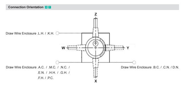
Connection Exit selected based on Draw Wire Enclosure **5**. When Connection Type is "Draw Wire Only" then Connection Orientation **6** is 0.
