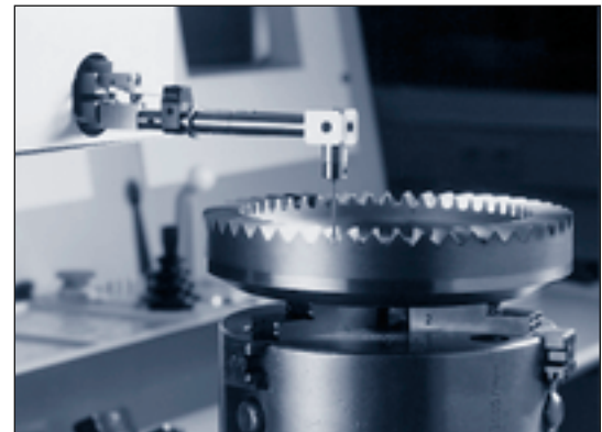
Computerized mapping of gear tooth profile
