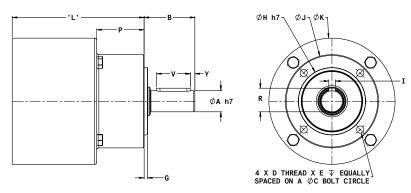
\* 'L' Dimension will change depending on motor being used. Note: Mounting adapters available for both round and square motors.
