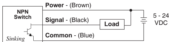
NPN wiring connection - both NC &amp; NO
