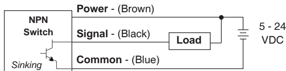
NPN wiring connection - both NC &amp; NO
