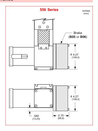
**Note:** This power-off electric brake MUST NOT be engaged when the positioning table is in motion. Moving the table with the brake applied could damage the brake and the positioning table. Also, continuous use of this brake to stop a table (load) that is in motion could damage the brake and the positioning table. Dynamic braking of a positioning table should be done by the motor and not the brake.
