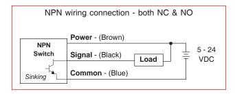
Standard *LINTECH* Wiring (provided when switch option is ordered with any table)
