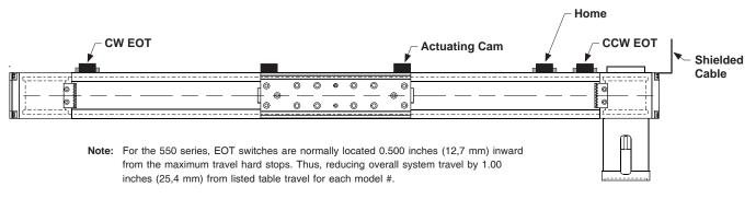
Note: Each switch can be located anywhere along the T-slots, which run on both sides of the table.
