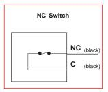
Standard *LINTECH* Wiring (provided when switch option is ordered with any table)
