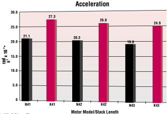
\* Holding Torque Rotor Inertia ...a figure of merit for acceleration capability
