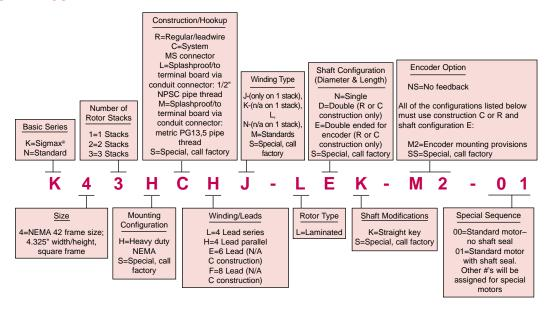
The example model number above indicates a K series (Sigmax®) NEMA 42 frame motor with a three stack rotor. This motor is equipped with a heavy duty front end bell and shaft, and a sealed system rear end bell with MS connectors. It also has a bipolar parallel connection, a J winding, a straight keyway, a shaft seal and encoder mounting provisions.
