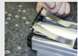
All DS4 and DS6 tables will bolt directly together in a standard XY without modification.
