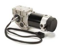
With a choice of output ratios, our MobilePower line of products helps power battery-operated vehicles from wheelchairs to lift trucks. And, to increase durability and decrease noise levels, the robust all metallic gears are hobbed to a precision AGMA 9-Class.
