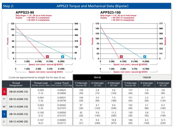
Motor step rate calculation: Motor step rate (halfstep/sec) = [Speed (in/sec)\*2] / [travel (in/fullstep)]
