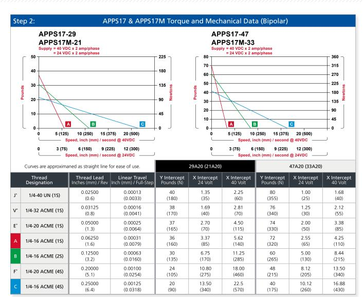
Motor step rate calculation: Motor step rate (halfstep/sec) = [Speed (in/sec)\*2] / [travel (in/fullstep)]
