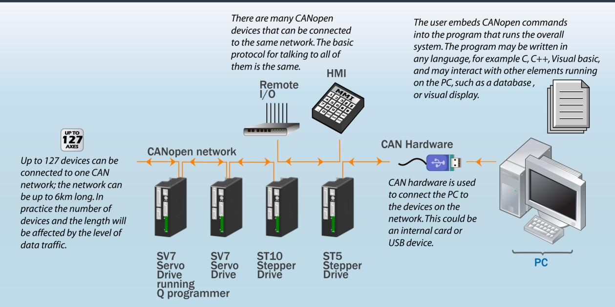
Different CANopen drives can be connected on the network, including ST and SV drives. AMP drives have the DS301 and DSP402 protocols implemented. All AMP CANopen drives have ANPSO Commer available to excecute Q sequences, these sequences can be modified and triggered via the CAN network. Toll Free Phone: 877-378-0249
