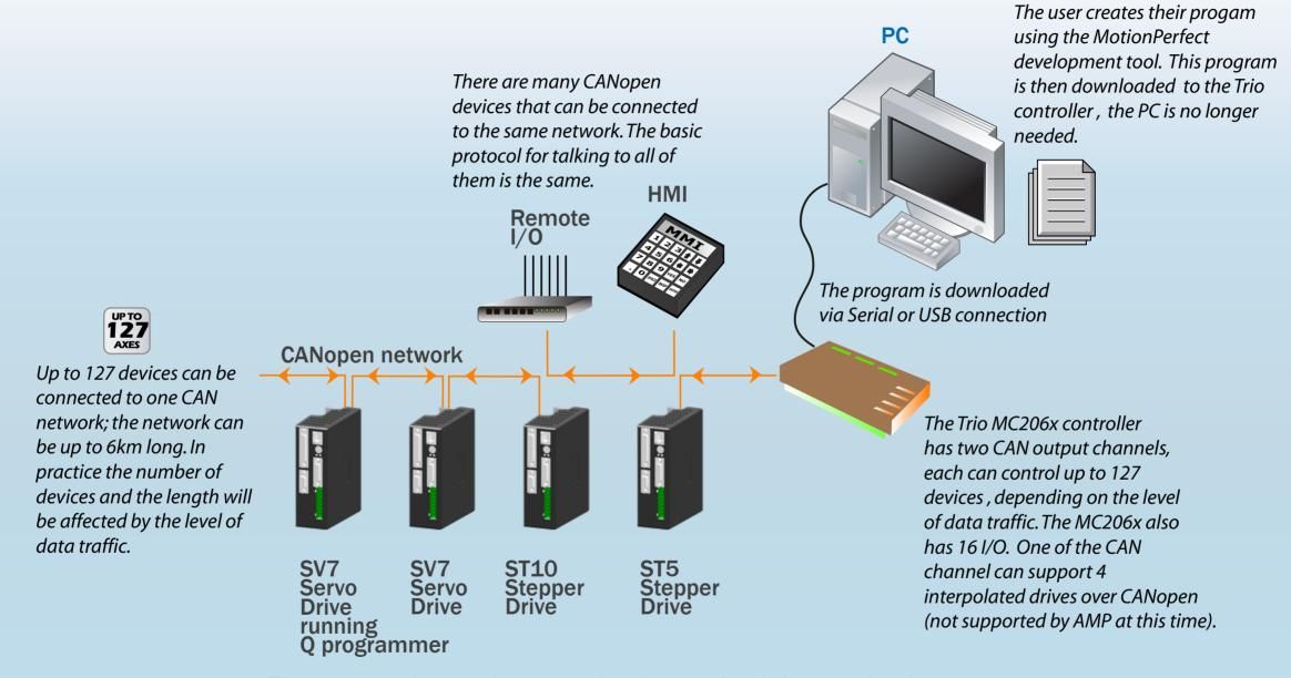
Different CANopen drives can be connected on the network, including ST and SV drives. AMP drives have the DS301 and DSP402 protocols implemented. All AMP CANopen drives have AMP's Q processory of a labele to excecute Q sequences, these sequences can be modified and traggered via the CAN network.
