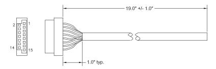
Half Meter Cable One End Terminated: 2081AG019 = 14 conductor 28 AWG for UVW Commutation 2083AG019 = 8 conductor 28 AWG for non-Commutation Connector = JAE FI-W15S
