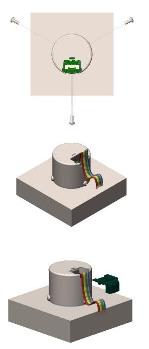
Slide housing over adapter plate. Secure housing by tightening the three M2.5 screws using a Philips screw driver with a torque of 0.4 Nm
