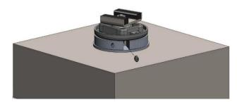
Tighten both set screws with a 1.3mm [0.05"] hex key, using the channel hole in the adapter plate with a torque of 0.5 Nm.
