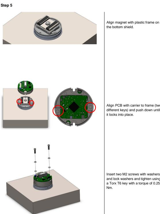
Align PCB with carrier to frame (two different keys) and push down until
