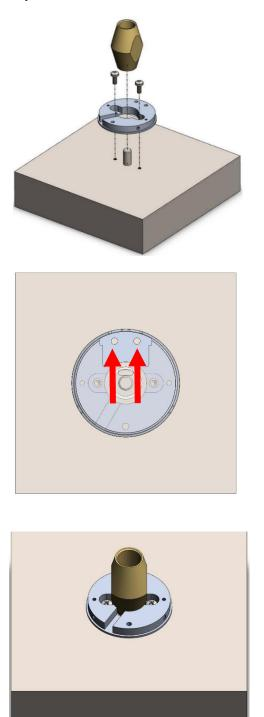
Slip adapter plate over shaft and use screws, depending on tapped holes in motor frame, to secure. Slip centering tool over shaft to center adapter plate to the shaft centerline.
