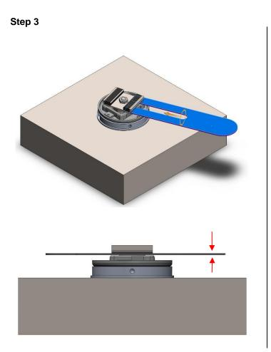
Slide gapping tool (Required thickness of 0.7mm [0.0275"]) between magnet and bottom shield. Push magnet down.
