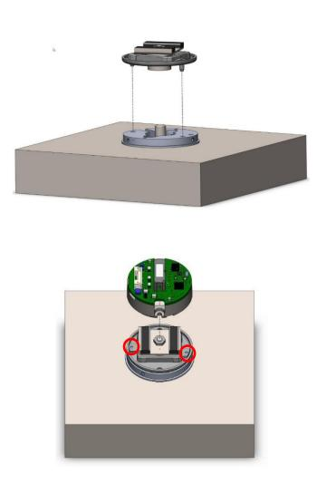
Slide bottom shield/magnet assembly over shaft and lock alignment pins into adapter plate. Push down bottom shield all the way so it lies flat on the adapter plate.
