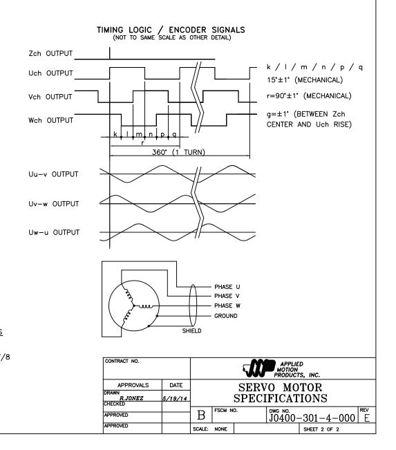
TIMING LOGIC / ENCODER SIGNALS
