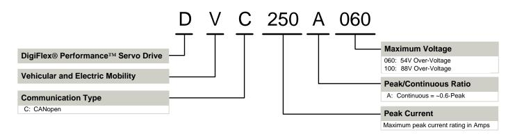
ADVANCED Motion Controls servo drives are available in many configurations. Note that not all possible part number combinations are offered as standard drives. All models listed in the selection tables of the website are readily available, standard product offerings.
