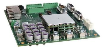
The **FD100-50-RM** is a serve drive and development board assembly for a FE100-50-RM FlexPro<sup>®</sup> series serve drive with IMPACT<sup>™</sup> architecture. Connections to the controller, motor, power, and feedback are simplified through the standard connectors featured on the board. The **FD100-50-RM** is ideal for prototyping and can be used in production and industrial environments as well.
