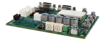
The **FD060-60C-RM** is a serve drive and development board assembly for a FE060-60C-RM FlexPro<sup>®</sup> series serve drive with IMPACT<sup>™</sup> architecture. Connections to the controller, motor, power, and feedback are simplified through the standard connectors featured on the board. The **FD060-60C-RM** is ideal for prototyping and can be used in production and industrial environments as well.
