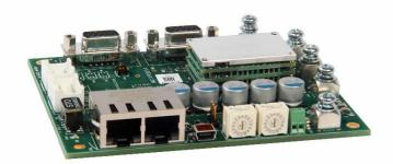
The **FD060-60C-EM** is a servo drive and development board assembly for a FE060-60C-EM FlexPro<sup>®</sup> series servo drive with IMPACT<sup>TM</sup> architecture. Connections to the controller, motor, power, and feedback are simplified through the standard connectors featured on the board. The **FD060-60C-EM** is ideal for prototyping and can be used in production and industrial environments as well.
