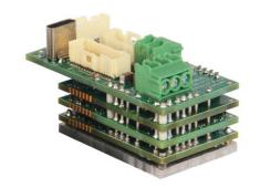
The **FXM060-5-EM** is an Extended Environment single-axis servo drive and integration board assembly for a FXE060-5-EM FlexPro<sup>®</sup> series servo drive with IMPACT<sup>TM</sup> architecture. Connections to the controller, motor, power, and feedback are simplified through the standard connectors featured on the board.
