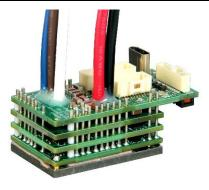
The FXM060-25-EM is an Extended Environment single-axis servo drive and integration board assembly for a FXE060-25-
