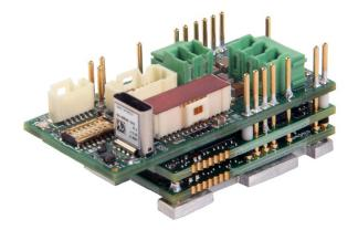
The **FM060-5-RM** is a single-axis servo drive and integration board assembly for a FE060-5-RM FlexPro<sup>®</sup> series servo drive with IMPACT<sup>TM</sup> architecture. Connections to the controller, motor, power, and feedback are simplified through the standard connectors featured on the board.
