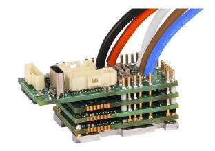
The **FM060-25-EM** is a single-axis servo drive and integration board assembly for a FE060-25-EM FlexPro<sup>®</sup> series servo drive with IMPACT<sup>TM</sup> architecture. Connections to the controller, motor, power, and feedback are simplified through the standard connectors featured on the board.
