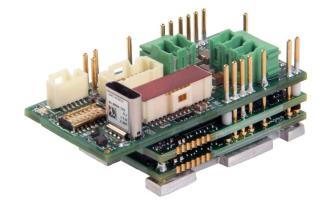
The **FM060-10-CM** is a single-axis servo drive and integration board assembly for a FE060-10-CM FlexPro<sup>®</sup> series servo drive with IMPACT<sup>TM</sup> architecture. Connections to the controller, motor, power, and feedback are simplified through the standard connectors featured on the board.
