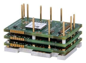
The **FE060-5-IPM** is a FlexPro<sup>®</sup> series servo drive with IMPACT<sup>™</sup> architecture.
