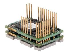
The **FE060-25-RM** is a FlexPro<sup>®</sup> series servo drive with IMPACT™ architecture.
