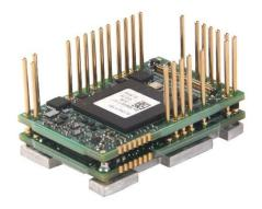
The **FE060-25-CM** is a FlexPro<sup>®</sup> series servo drive with IMPACT™ architecture.
