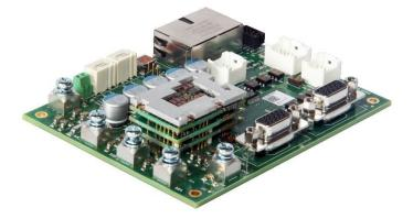
The **FD060-5-EM** is a serve drive and development board assembly for a FE060-5-EM FlexPro<sup>®</sup> series serve drive with IMPACT<sup>™</sup> architecture. Connections to the controller, motor, power, and feedback are simplified through the standard connectors featured on the board. The **FD060-5-EM** is ideal for prototyping and can be used in production and industrial environments as well.
