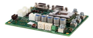
The **FD060-25-RM** is a serve drive and development board assembly for a FE060-25-RM FlexPro<sup>®</sup> series serve drive with IMPACT<sup>™</sup> architecture. Connections to the controller, motor, power, and feedback are simplified through the standard connectors featured on the board. The **FD060-25-RM** is ideal for prototyping and can be used in production and industrial environments as well.
