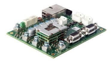
The **FD060-25-EM** is a serve drive and development board assembly for a FE060-25-EM FlexPro<sup>®</sup> series serve drive with IMPACT<sup>™</sup> architecture. Connections to the controller, motor, power, and feedback are simplified through the standard connectors featured on the board. The **FD060-25-EM** is ideal for prototyping and can be used in production and industrial environments as well.
