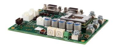
The **FD060-10-RM** is a servo drive and development board assembly for a FE060-10-RM FlexPro<sup>®</sup> series servo drive with IMPACT<sup>TM</sup> architecture. Connections to the controller, motor, power, and feedback are simplified through the standard connectors featured on the board. The **FD060-10-RM** is ideal for prototyping and can be used in production and industrial environments as well.
