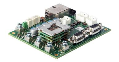
The **FD060-10-EM** is a servo drive and development board assembly for a FE060-10-EM FlexPro<sup>®</sup> series servo drive with IMPACT<sup>TM</sup> architecture. Connections to the controller, motor, power, and feedback are simplified through the standard connectors featured on the board. The **FD060-10-EM** is ideal for prototyping and can be used in production and industrial environments as well.
